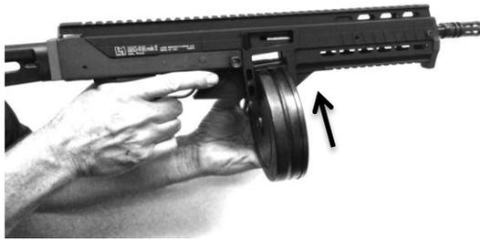
Due to variations in magazines, some magazines may be a snug fit but most will fit loosely. The magazine may have a lot of play after installation, but this will not affect functioning of the MAX-31A mk2.
