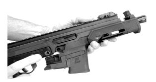
(5) Align retaining pin hole of lower receiver, upper receiver, and Magazine Module and install retaining pin.
