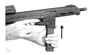
Due to variations in magazines, some magazines may be a snug fit but most will fit loosely. The magazine may have a lot of play after installation, but this will not affect functioning of the VERSA-12.
